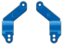
Aluminum axle carriers installed as labeled: 4 degrees toe-in
